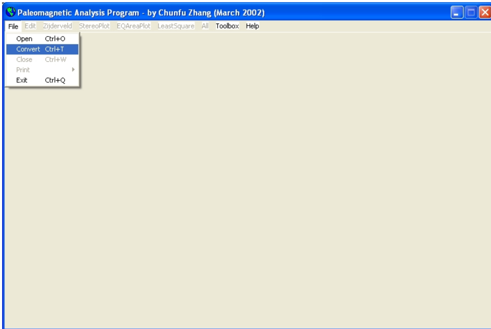
Figure 2 If you don't have a *.mag file but have suitable *.app, *.tab, *.cma, or *.txt files, you can select this F ile>Convert menu (or press Ctrl + T) to convert a desired file. For detailed file format, please refer to Help > Main Features (or press F1 key) or the PaleomagHelp.doc file.
