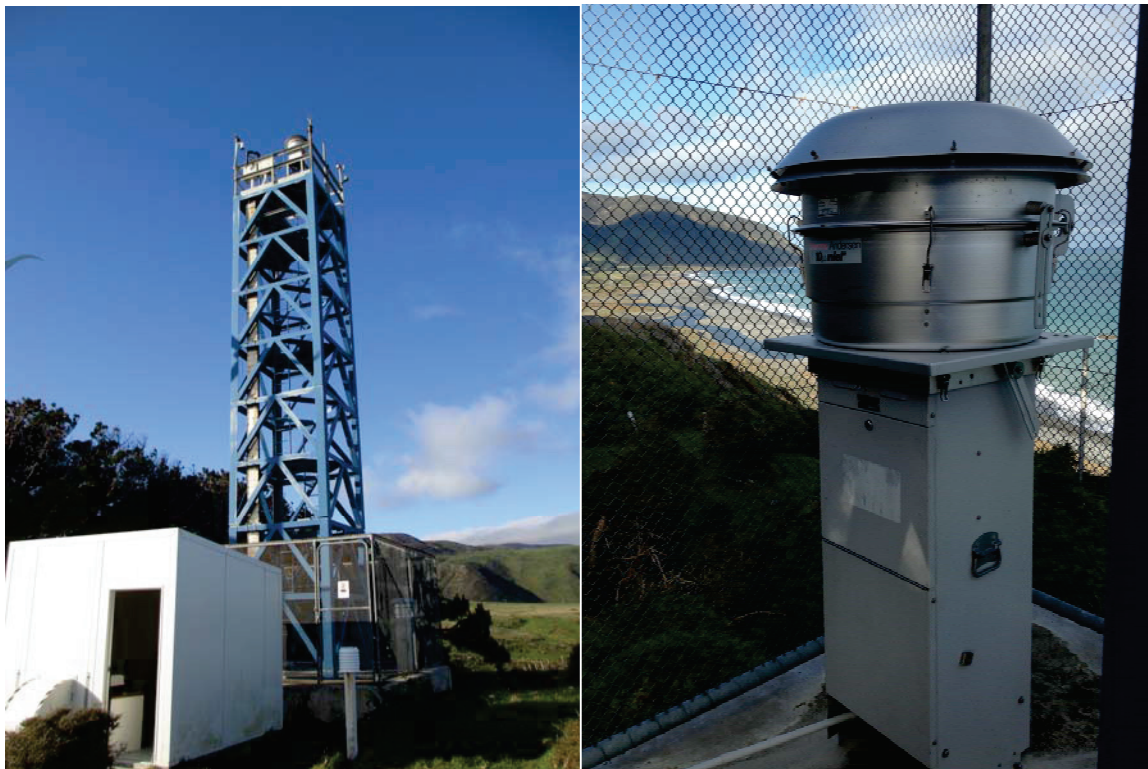
Figure A.6: The 15 m tower located at Baring Head (left) will have one sampler at the top and one at the bottom. A previously installed Lear Siegler sampler with PM10 inlet at the top of the tower will sample only southerly events. A second sampler, installed at the base of the tower (right) during EAPSI, will continuously sample all air masses.
